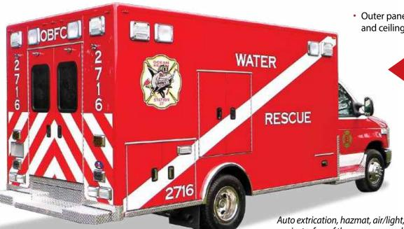
Outer panels, exterior compartment walls, and ceilings are .125" aluminum
